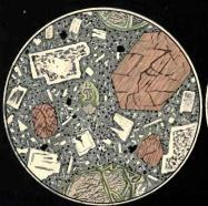
Fig. 3. Porphyritic Basalt. Lion's Haunch, Arthur's Seat, × 15.
